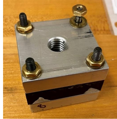
Figure 15. Aluminum block bolted to ABS block (Note: all tested samples had two nuts per bolt)
