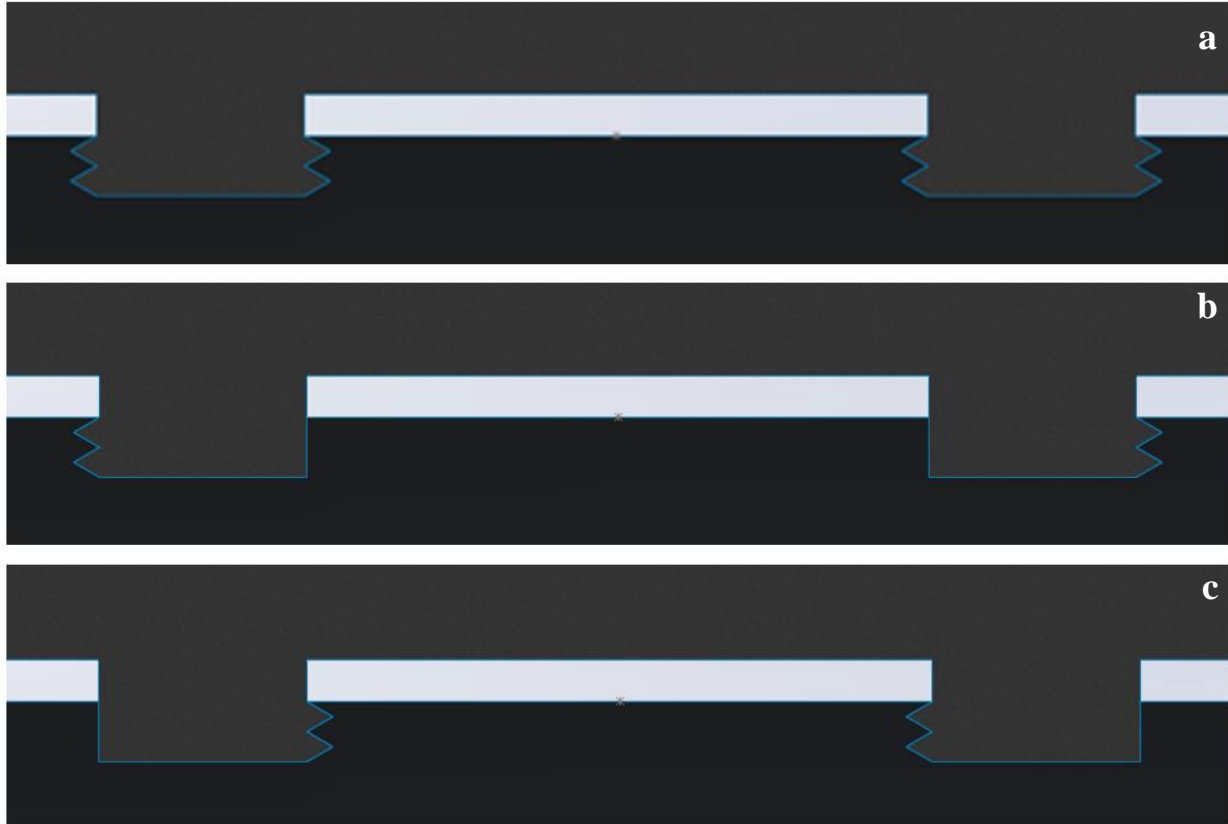
Figure 45. (a) Dual threads vs. (b) exterior threads vs. (c) interior threads
