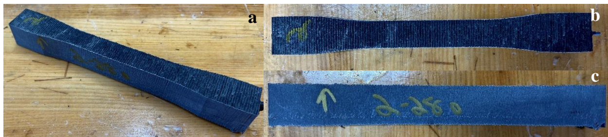
Figure 6. Tensile bar prior to machining in (a) isometric (b) top and (c) left side view
